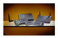
802.11b – Transmits at 2.4 GHz, sends data up to 11 Mbps using direct sequence spread spectrum modulation. 100 -150 feet range
