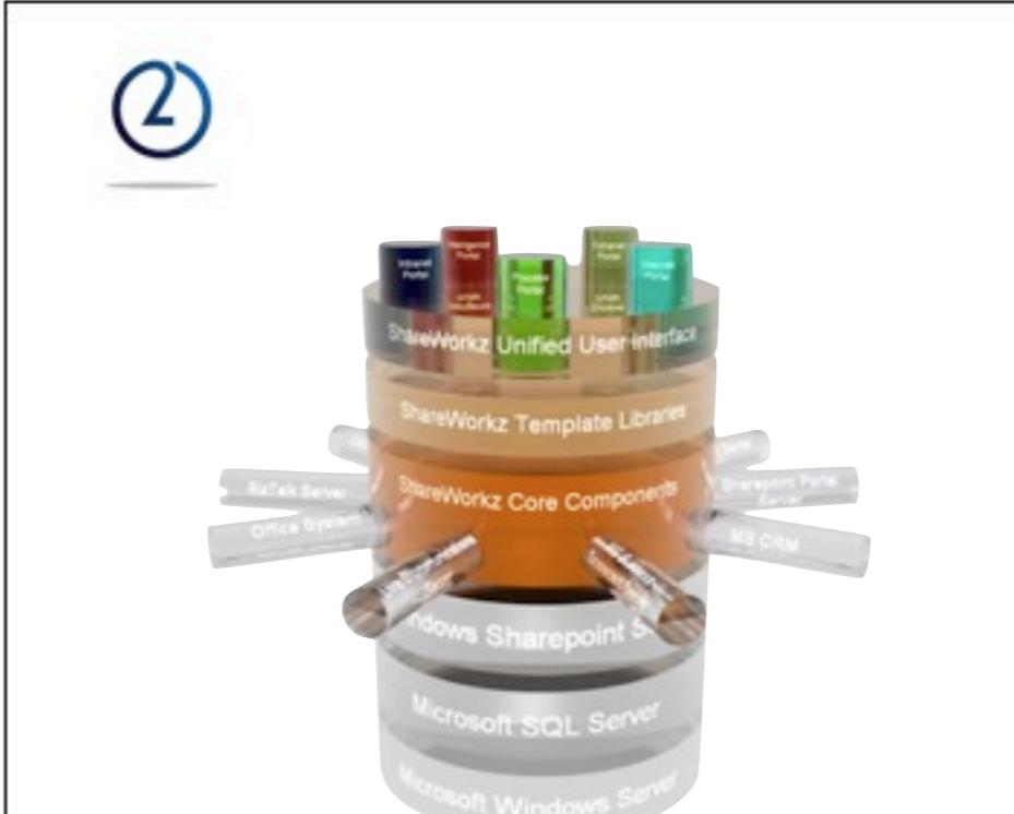
The diagram illustrates the ShareWorkz architecture as a layered system. At the bottom is Microsoft Windows Server. Above it is Microsoft SQL Server. The next layer is Windows SharePoint Server, with ShareWorkz Core Components integrated into it. Above this is ShareWorkz Template Libraries, and the top layer is ShareWorkz Unified User Interface, which includes various modules like Visual Portal, Business Rules, Business Logic, Business Data, and Business Forms.
